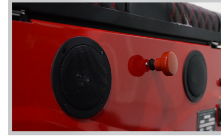
Electrical Emergency Stop Button Acil Elektrik Kesici Buton
